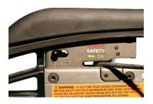
2) Loosen the T knob which locks down on the steel wedge on your Crossbow Defuser.
