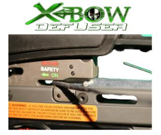
5) Pointing in a safe direction, take the safety off and squeeze the trigger. You will hear a click. Your serving is now being supported by the Crossbow Defuser. Holding the crossbow by the foregrip with one hand, and pointing in a safe direction, unscrew the T knob with your dominant hand until the string and serving are in the defused/neutral position. Unscrew the T knob just slightly more, slide back 1/2", tighten, and lift off.
